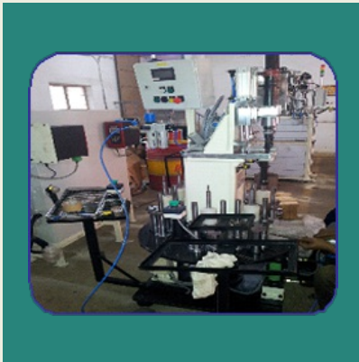
Industrial 3 Station Limb Assembly Machine
