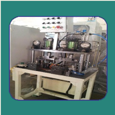
Industrial 3 Point Caulking
