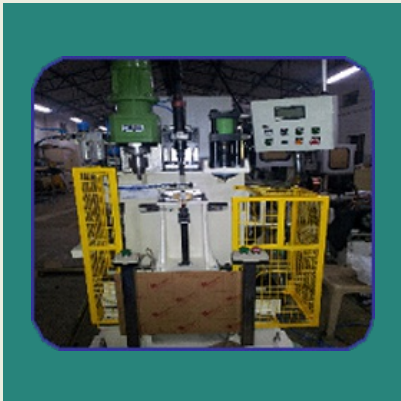
Industrial 3 Station, Torquing & Spin Riveting
