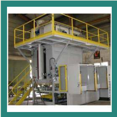
Industrial Heat Treating Vertical Oven
